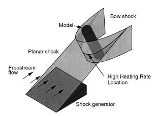
Fig. 2 Experimental setup shows where the planar shock and bow shock will intersect and produce the high heating rates.
