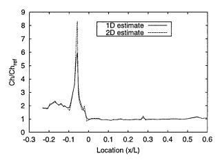
Fig. 6 Comparison of two-dimensional and one-dimensional estimate of Macor-2 at 2 s.
