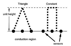
Fig. 3 Triangular patch provides a linearly varying function in space for sensitivity calculations, whereas the constant patch provides simple implementation but too much bias.
